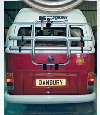
Bike rack (with spare wheel in car) or towbar mounted version for vehicles with rear wheel carrier
